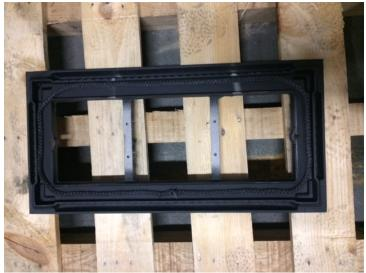
Top Casting rope gasket detail
