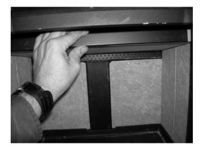
9) Place the bottom refractory stones into the stove.
