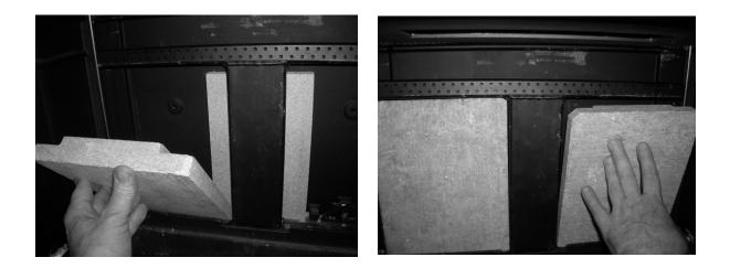
5) Place the left and right stones into the stove, exactly as shown-with the cut portion up and facing into the firebox.
