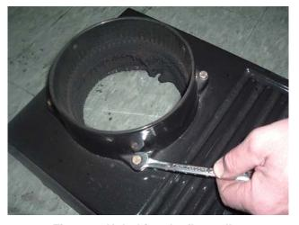
Figure 1: Unbolting the flue collar
