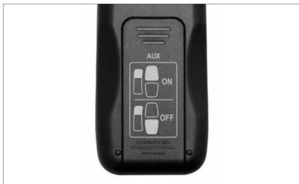
Figure 46 – Aux Burner Control Instructions
