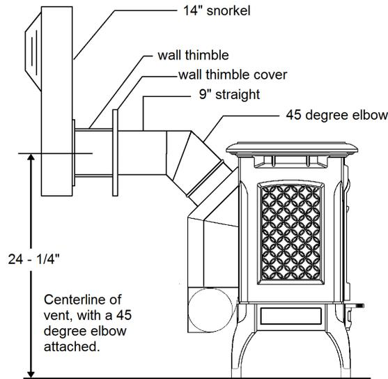
**Figure 9 - Components for a Typical Snorkel Installation**
