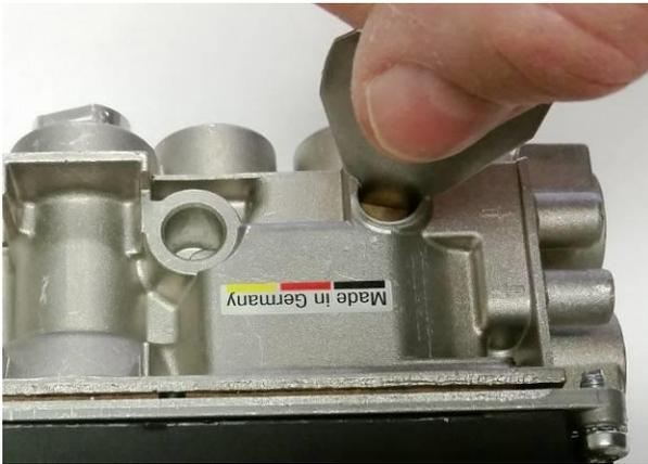
**Figure 26 – Tighten LP Low Flow Orifice**
