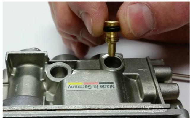
Figure 24 – NG Low Flow Screw Removal
