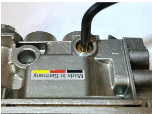
Figure 22 – Low Flow Orifice Removal
