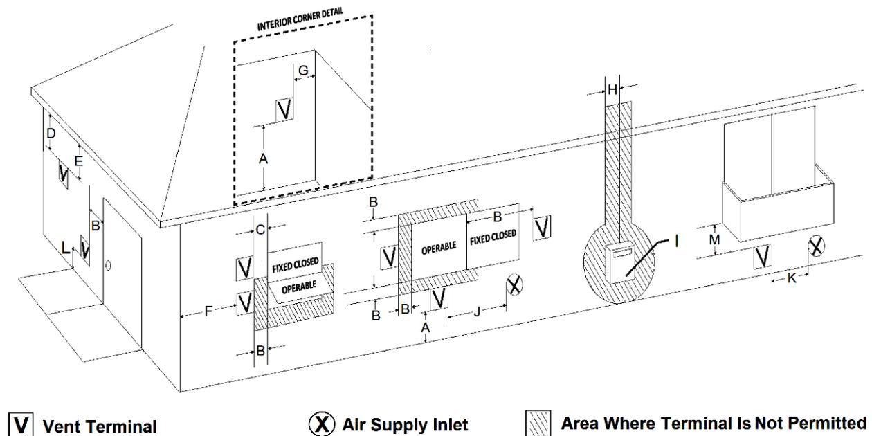
**Figure 12 - Acceptable Direct Vent Terminal Vent Cap Locations**
