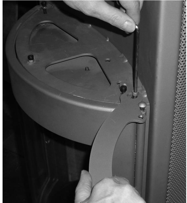
Figure 2 – Door Assist Tool pt# 5180-002
