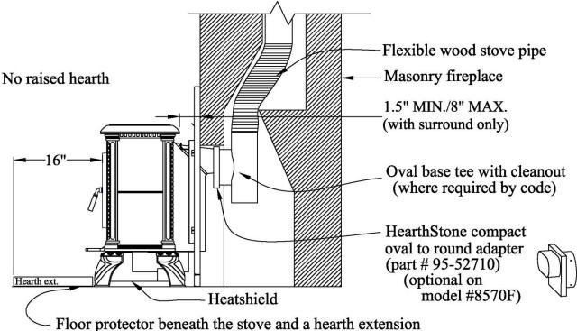
Floor protector beneath the stove and a hearth extension with an "R"-value of 2.5 or listed to U.L. 1618, extending 16" in front of glass and 8" beyond either side of the fuel and ash door openings.
