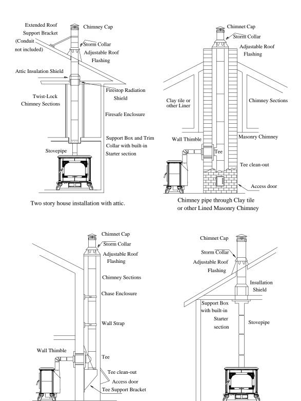
Chimney through outer wall with enclosed chase. Chimney is supported by Tee Support Bracket. One story house installation with attic. Chimney is supported by Ceiling.
