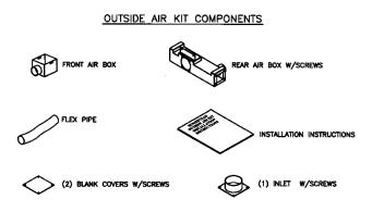
The Outside Air Kit allows for a direct stove connection of a 3" (76 mm) diameter duct (which you can obtain from another manufacturer); this duct leads to the outside of the house. Connect the duct to your stove in a number of ways (illustration is typical for both Hearth Mount and Freestanding models). Choose the one that is most convenient.
