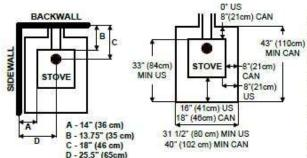
When installed on a combustible floor, non-combustible floor protection is required to cover the area beneath the heater, and extend at least 1817-41cm) [187 (48cm) CAN) to the front and 87/21cm) beyond each side of the fuel loading and ash removal openings [side of stove in CAN), the floor protection must extend under the flue connector and extend 2" beyond each side of pipe.
