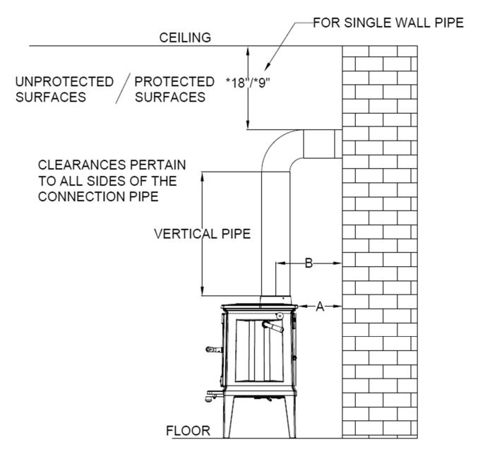
**Figure 5 Chimney Connector Clearances**
