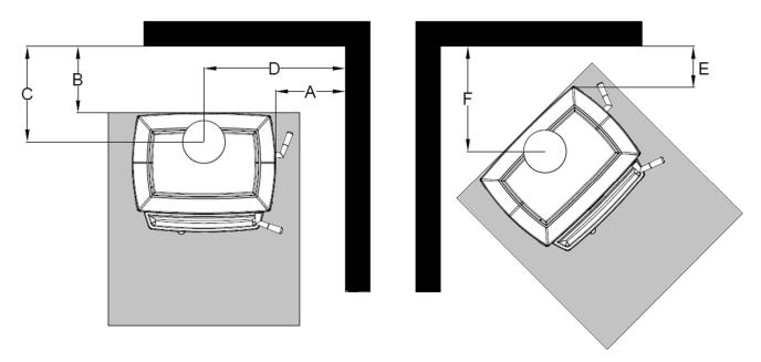
Figure 4 – Clearance to Combustibles
