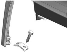
Figure 10 - Lock Down Detail
