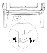
Figure 17 – Air Control Position
