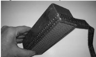
12. Wrap the gasket tape around the catalysts so it is reasonably tight. Double layer the material on three sides of the individual catalyst cartridges as shown in the following picture.
