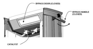
Figure 14 - Bypass Closed
