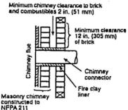
Minimum chimney clearance from masonry to sheet steel supports
