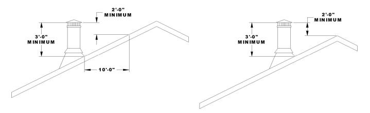
**Figure 8 Chimney Height Requirements**
