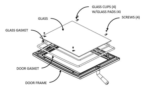
Figure 22 - Front Door Assembly
