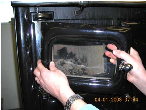
Slightly lean the firebox door so that you can lift it off the bottom hinge pin.
