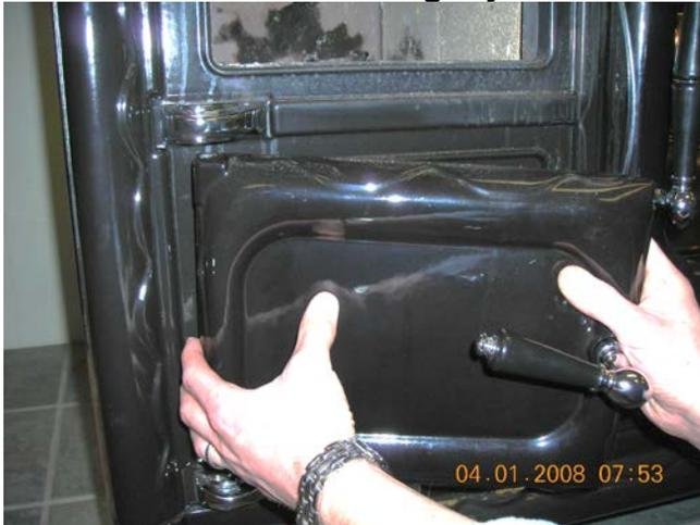
**You now have access to the lower pin for the ash door, if necessary.**
