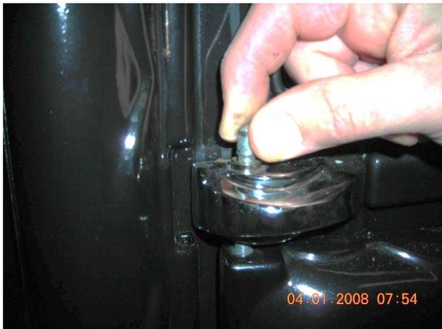
Now lift out the pin from the lower hinge on the firebox door. This is also the pin in the top of the ash door.
