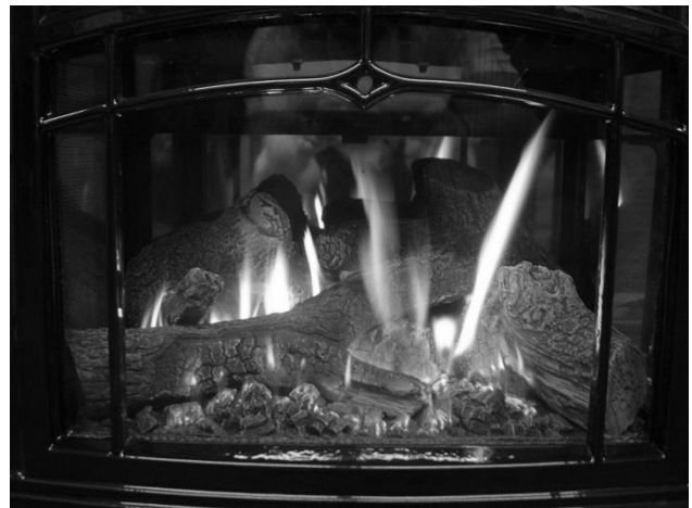
Photo 9 – Typical Burner Flame Appearance
